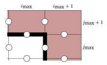
Figure 3. The thicker line is the boundary, and the shaded cells are the boundary strip. The circles represent the sampling positions. Notice that some points on the boundary are not sampled, hence the need for a boundary strip.
