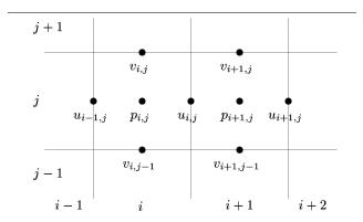
Figure 2. Staggered grid discretization.
