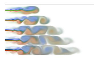
Figure 1. A  $1024 \times 128$  Navier-Stokes simulation running at interactive rates, Re = 10000.
