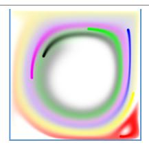
Figure 8. Lid-driven cavity,  $256 \times 256$  grid, Re = 10000. The counter-eddies in the corners are experimentally confirmed for large Re.
