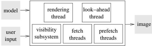
Figure 7: The rendering architecture.
