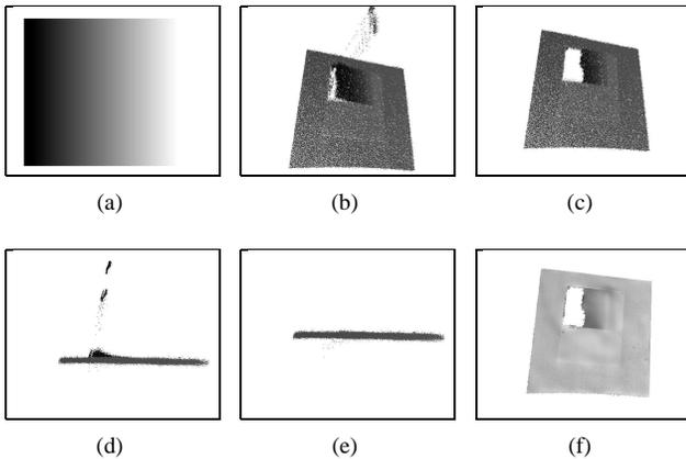
Figure 4: Removing intensity bias. (a) Test pattern. (b) Before removing bias. (c) After removing bias. (d) Side view before. (e) Side view after. (f) Reconstructed surface.
