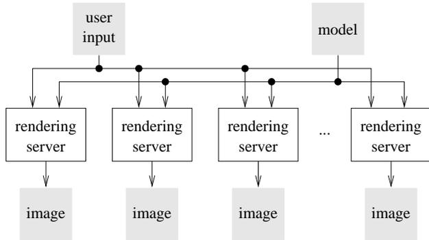
Figure 8: The parallel rendering architecture.
