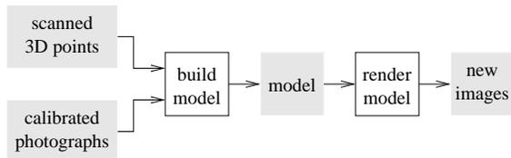
Figure 1: Our acquisition and rendering pipeline.
