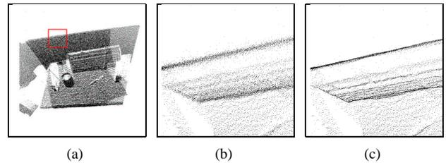
Figure 5: Removing noise. (a) Scan of a desktop. (b) Before removing noise. (c) After removing noise.
