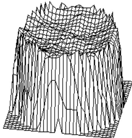
Figure 8- MAP Filtered Reconstruction - Beta distribution - Simulated Phantom
