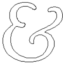
Figure 4: Example of a Cooper font composed of 22 Bézier curves.
