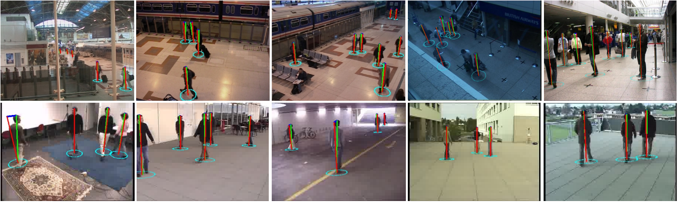
Fig. 8. Examples of camera auto-calibration results. Green line segments represent the ground truth manually labeled; Red line segments represent the estimated feet-head projection; Cyan circles represent the person position at the ground plane. The first row contains images from PETS 2006 (the first three) and from PETS 2007 (the last two). Second row contains images from CVLAB data set.
