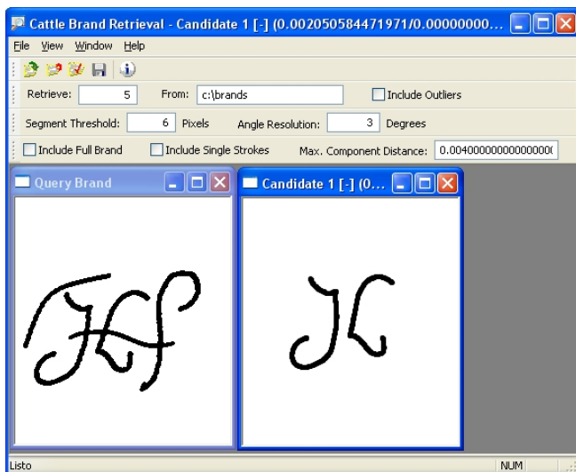
Figure 8. Example case: The exclusion measure for the query F and database brand G yields M(F, G) = 0.00 , the value for the distance between the only matching pair components is \|x_i - y_i\| = 2.05 \times 10^{-3} .
