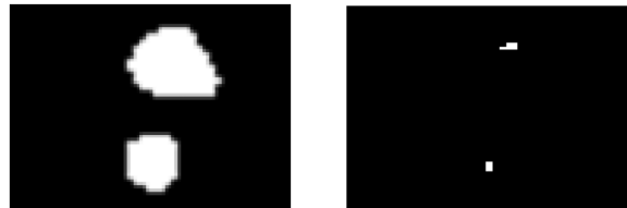
Fig. 3. Object marker creation: Ultimate erosion onto binarized prediction weights. The image on the left represents the activation map after binarization, where we applied a threshold to select as objects the set of pixels with the highest prediction weights ( grayscale value > 100). The image on the right is the result after the ultimate erosion procedure, using the binarized image as input.
