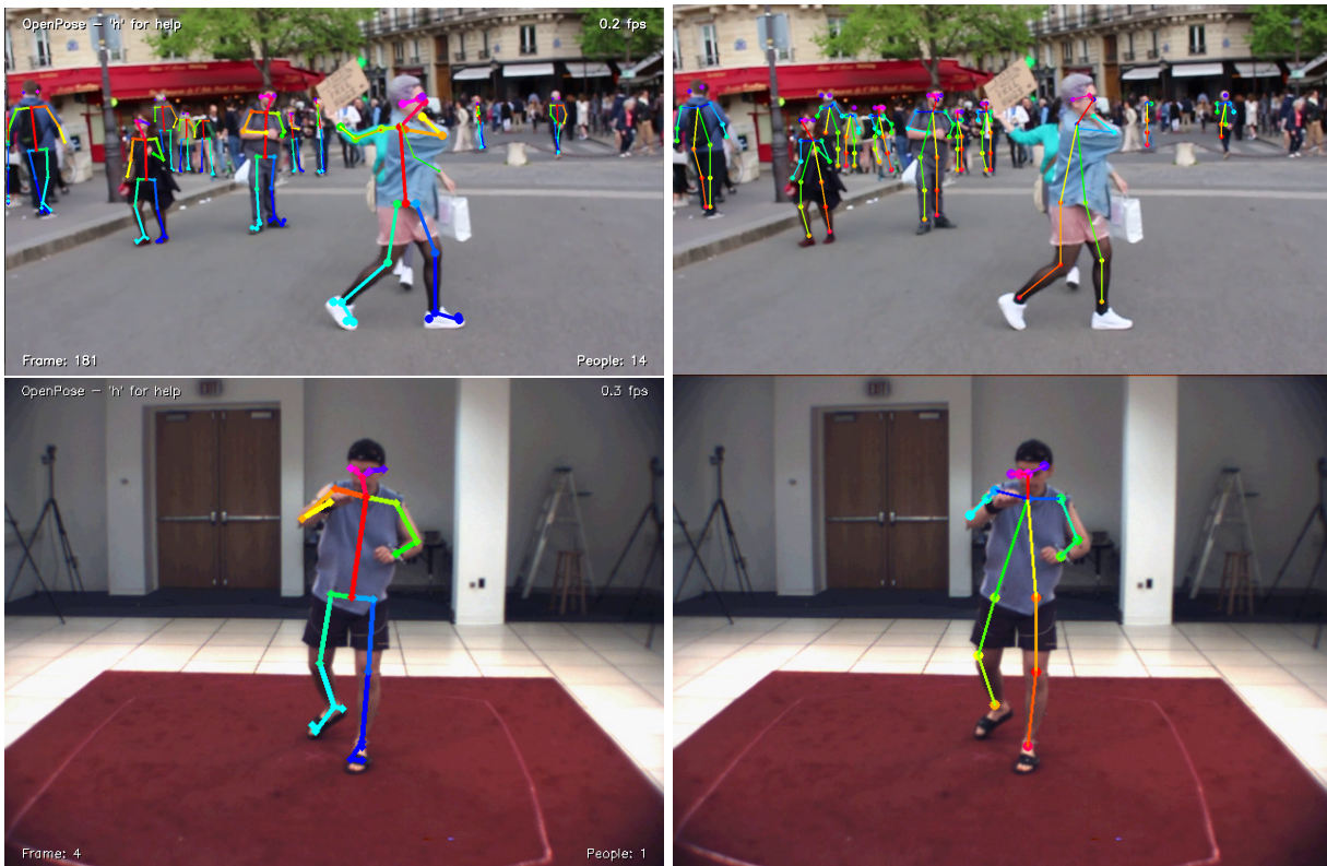
Fig. 3. Comparison between the OpenPose model and ours. The first figure (left) is generated by the OpenPose and the second by our model (right). As we can see, our model is slightly less accurate than the original work in particular cases, considering the exact position of a keypoint. Although, OpenPose presents a confusion between semantically similar parts of different persons in this frame. Also, our model do not consider all the feet keypoints.
