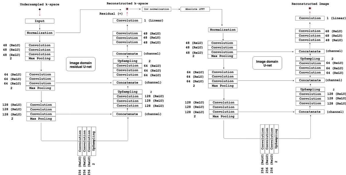
Fig. 2. Architecture of our hybrid model. The k-space network uses a  $5 \times 5$  convolution kernel size and the image domain network uses a  $3 \times 3$  kernel. Due to its topography consisting of two U-Nets, we term this hybrid method a W-Net.
