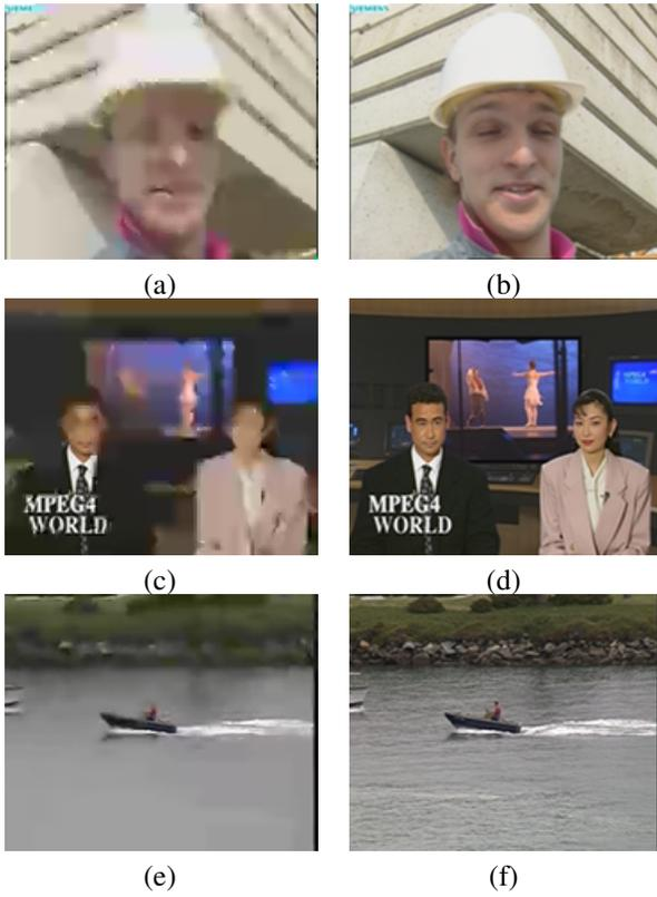
Figure 4: Frames extracted from the *Foreman* (a – b), *News* (c – d) and *Coastguard* (e – f) sequences, respectively; (a), (c) and (e) represent degraded versions (i.e., base layer-only decoding), while (b), (d) and (f) represent the full-quality versions.
