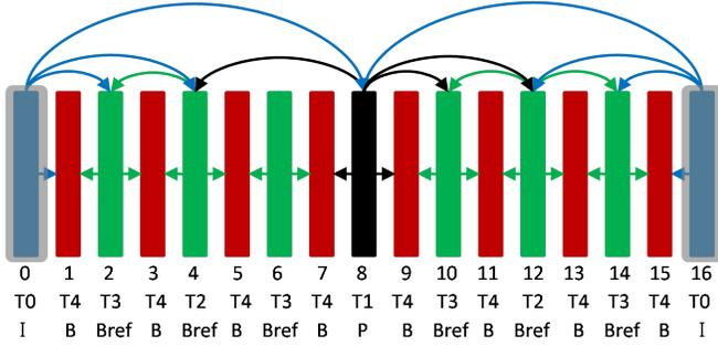
Figure 8: *Best* approach - only I frames, highlighted in gray, have enhancement layer bits encrypted with AES.
