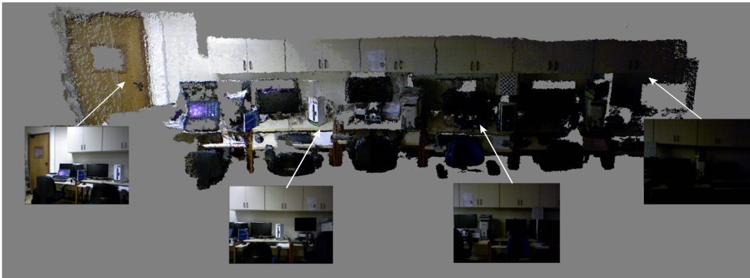
Fig. 1. Registration of a partially illuminated scene, a hard task due to the lack of textural information. The cloud alignment was done using the proposed RGB-D descriptor, Binary Appearance and Shape Elements (BASE), that combines appearance and shape.
