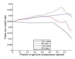
Fig. 2. Error versus reject curves for Zhaos approach [10]. The threshold is set to give an initial false non-match rate of 2.5%. The black, red and blue solid lines indicate, respectively, the OCL, Mu, and LCS quality indexes, while the black dashed line indicates the response of the OF quality index.
