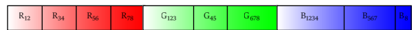
Fig. 2. Our modelling implements each individual as a binary array, being one value for each colour tonality interval. If a interval has its respective bit as set, it has its own position in the produced quantization, otherwise, it is aggregated to the immediate previous interval.
