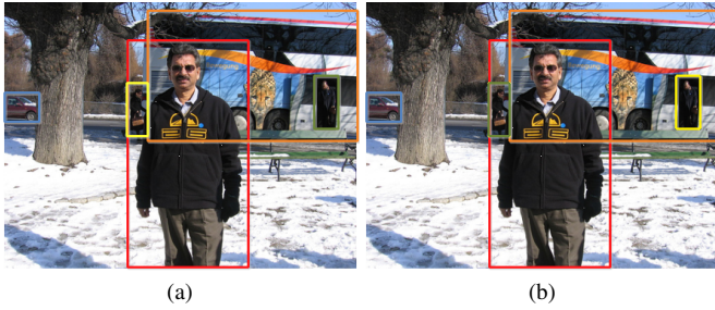
Fig. 9. EIRA importance output and corresponding ground-truth. The color of the boxes indicate the importance, the reddish colors show higher importances. (a) EIRA importance output; (b) annotated importance ground-truth (better viewed in colors).
