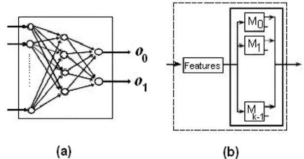
**Figure 10. Class-modular architecture [11]: (a) sub-network and (b) whole network with  $K$  modules.**
