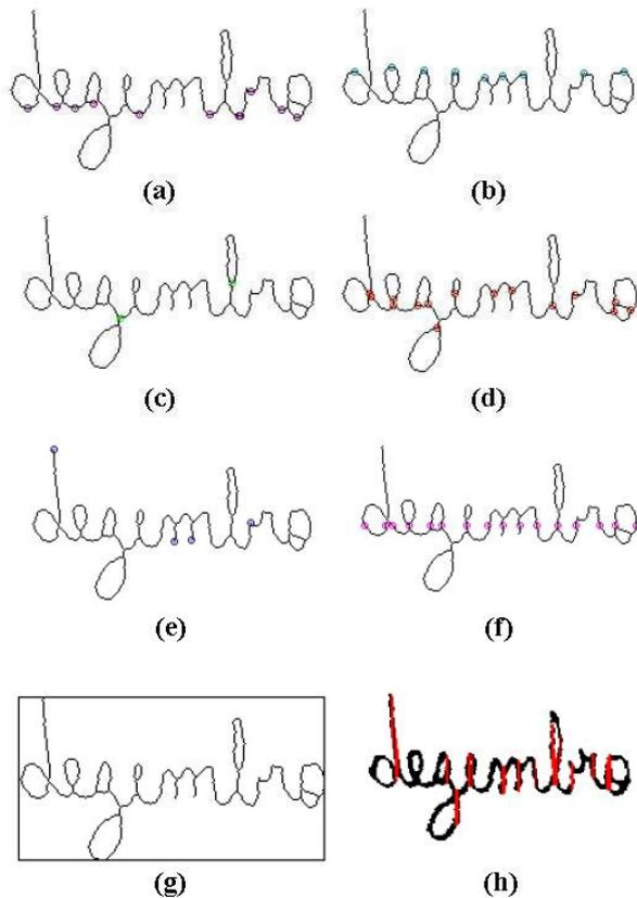
**Figure 9. Feature extraction: a) concave semicircles, b) convex semicircles, c) crossing-points, d) branch-points, e) end-points, f) NCH, g) NPP and h) vertical lines.**
