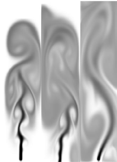
**Figure 10. Smoke simulation with large  $Re$ .  $128 \times 1024$  grid,  $Re = 10000$ , inflow in the south, outflow in the north.**
