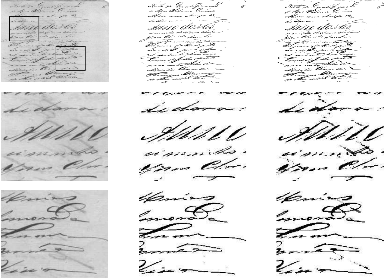
(a) Original image (b) Proposed operator (for k = 5 and \sigma = 0.3 ) (c) Moving average algorithm
